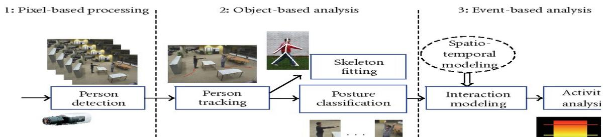
Fig. 1 Block diagram of the Behavior Analysis Algorithm
